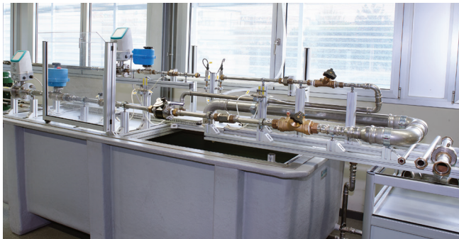
Flow Loop testing facility
