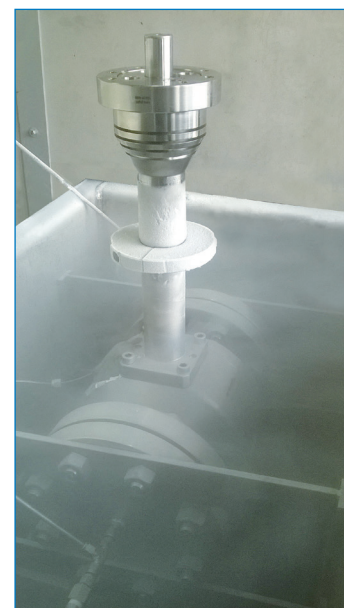
Fig. 8 - Split Body cryogenic valve under testing
